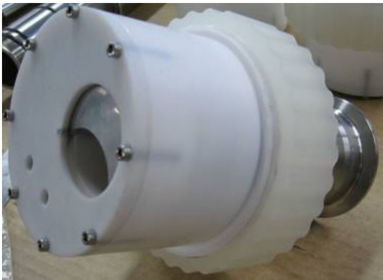
Figure 4 Vessel lid with shutter and an two gas outlets
